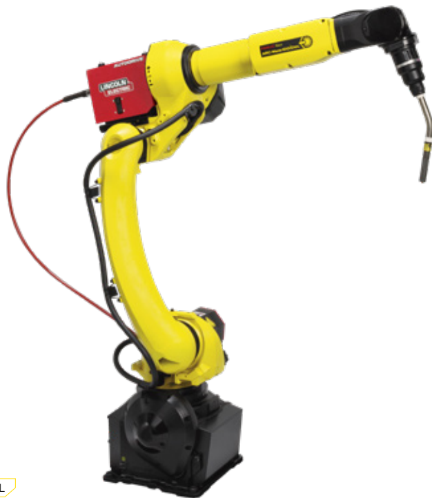
ARC Mate 100iD/10L Long arm, hollow wrist
