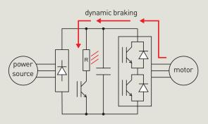
FANUC's state-of-the-art AC drive systems use high-speed, high-efficiency switching circuits to direct the energy back into the main electrical supply, reducing the net energy used. When combined with the more efficient motion processes provided by the Power Motion *i*-MODEL A, electricity costs can be reduced significantly.
