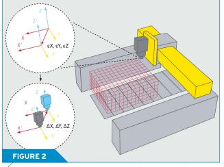
3-D error compensation applied directly in the work space.
