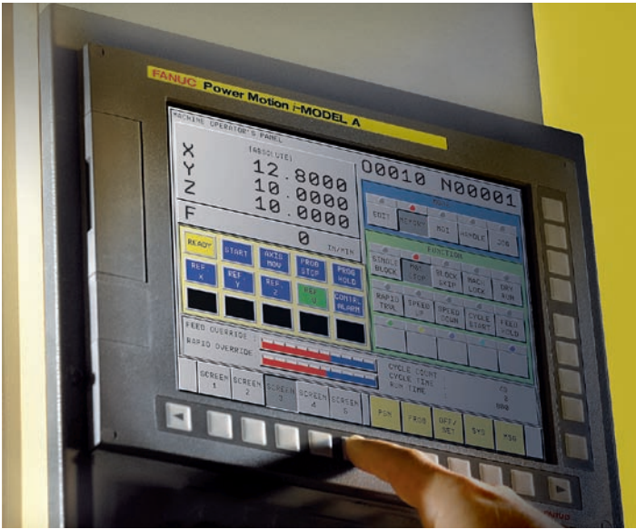
A solution for motion control challenges is the new FANUC Power Motion i-MODEL A introduced at FANUC's recent Open House Show at its headquarters at the base of Mt. Fuji in Japan. It is suited for a wide range of multi-axis and multi-path functions for motion control applications.
