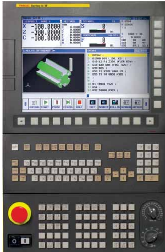
Close-up of the FANUC Series Oi-TF CNC.
