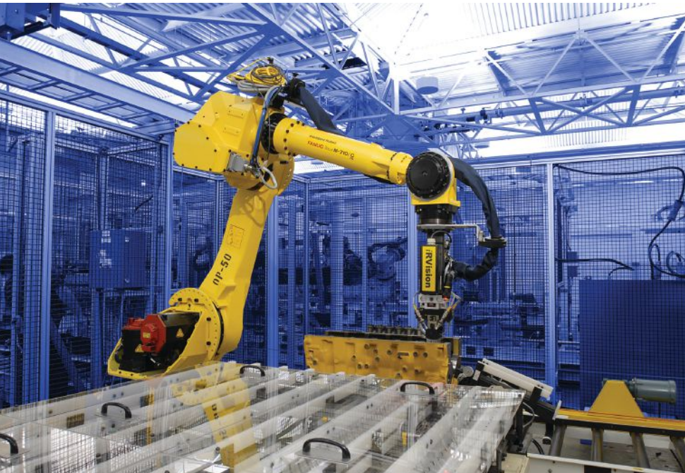
'Critical-path' components drive cell design and integration. A robot-guided process that relies completely on the machine vision implementation. Source: FANUC America Corp.
