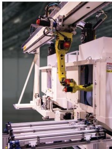
Today's flexible automation systems demand increasingly higher levels of systems integration skills. A multi-station machining cell with automated robotic load and unload. Source: FANUC America Corp.
