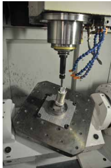
Acquiring a table-rotation five-axis machining center focused the shop's attention on the value of the CNC programs that could run on either type of machine. Vector programming makes this possible.
