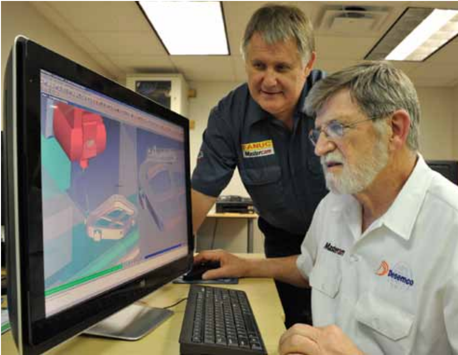
Grant Salmon looks over Dave Watson's shoulder as he checks the simulation of a five-axis machining operation. Desemco uses Vericut software extensively to verify and optimize five-axis CNC programs created by Mastercam.
