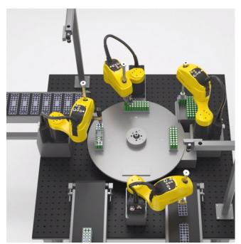
SR-3iA SCARA Robots assembling battery packs
