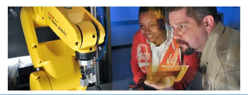
**ER-4iA Fenceless -** The FANUC ER-4iA fenceless education cart combines FANUC's DCS position and speed check software with a mini safety laser scanner. FANUC's fenceless cart fits through a standard door and runs off 110V power. The fenceless cart provides a larger work envelope and introduces students to FANUC's and Allen-Bradley's integrated safety products.
