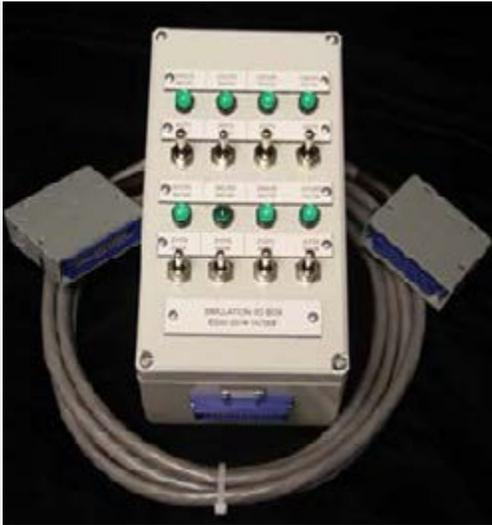
**I/O Simulator Box** - FANUC America's Industry Certified Education Robot Training program offers an I/O Simulator Box - Designed to give students an application to use digital inputs and outputs. This plug and play unit has eight digital inputs and eight digital outputs.
