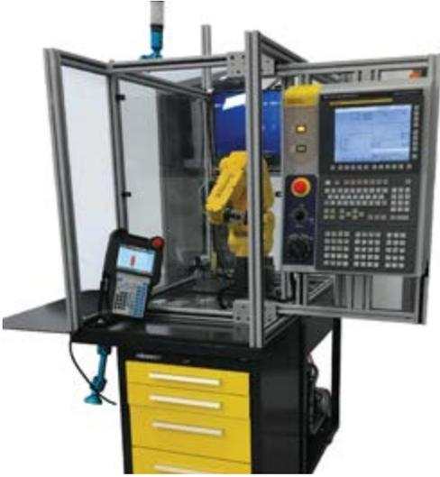
**Machine Tending Educational Cell (MTEC)-SIM** - The Machine Tending Education Cell Simulator (MTEC-SIM) is a feature-rich robot and CNC self-contained training cell for multi-level FANUC certifications.
