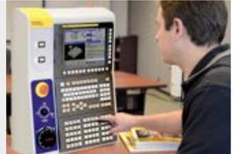
**Machine Simulator** - With a realistic machining simulation function, users can virtually manufacture parts in milling or turning environments with realistic kinematics and structure. The simulation is based on actual CNC position data, not on the G-code program, providing the most realistic simulation as the virtual machine reacts exactly as a real machine would.
