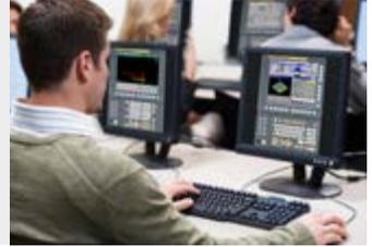
**CNC Simulator** - Students will experience the look, feel and layout of the control as they navigate and program a fully functioning CNC without the need for a full machine. This simulator is based on the FANUC Series 0i-MODEL F platform and can be operated in either milling or turning configurations.
