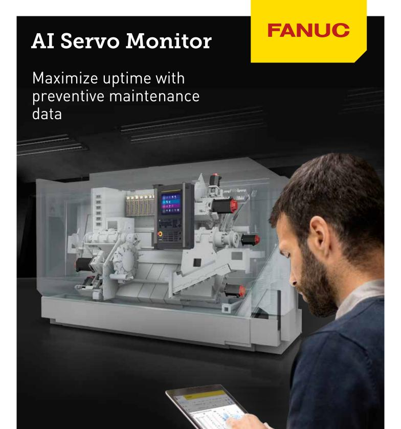
Al Servo Monitor is a software that visualizes anomalies of drive systems for servos and spindles through machine learning. Daily processing data is analyzed and displayed in easy-to-read, intuitive graphs.
