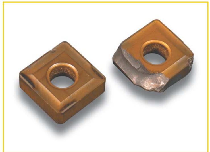
*Figure 16. Premature and uneven tool wear possible when tool is not loaded consistently.*
