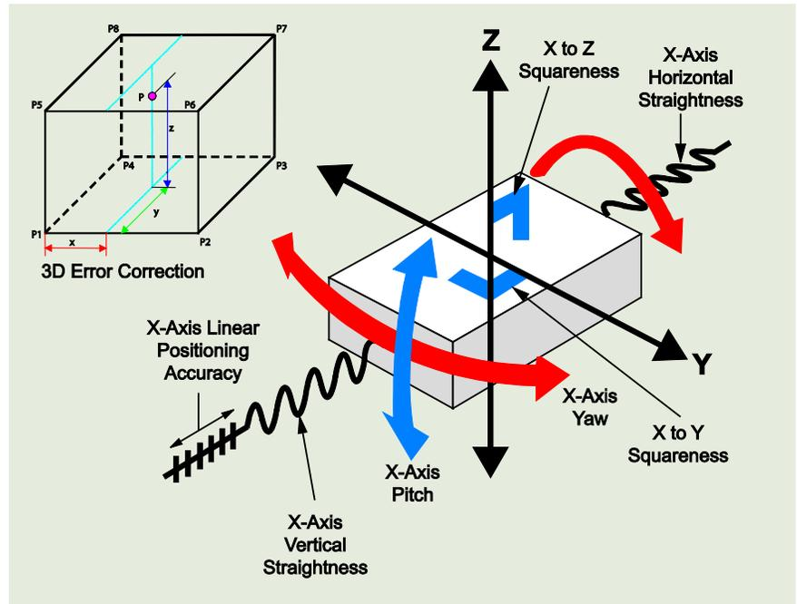
Figure 14. Degrees of freedom and common errors that can be compensated with 3D Error Correction
