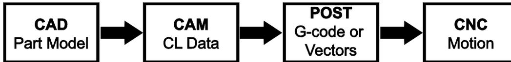
At a first glance, there appears to be very little difference between the part-centric workflow and the machine-centric workflow. Indeed the first two elements are identical. The 5-axis part-centric workflow also has four elements:
