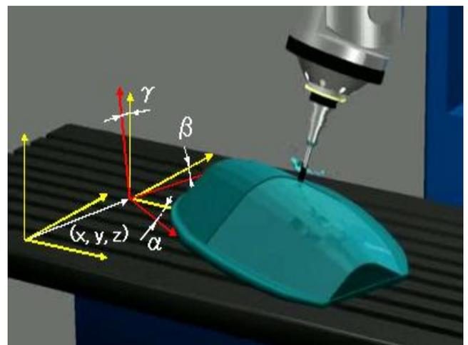
Figure 6. The CNC compensates for position and orientation of the part on the table.
