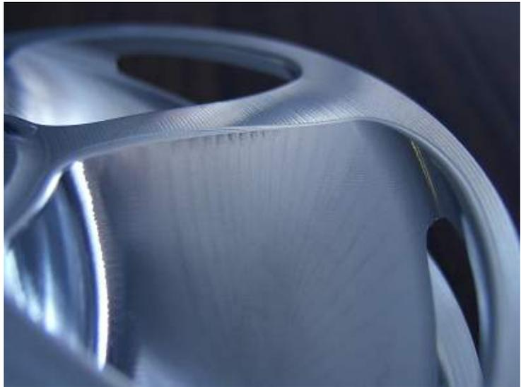
*Figure 2: Stripes on the machined surface due to point-to-point linear segment programming and machine vibrations.*
