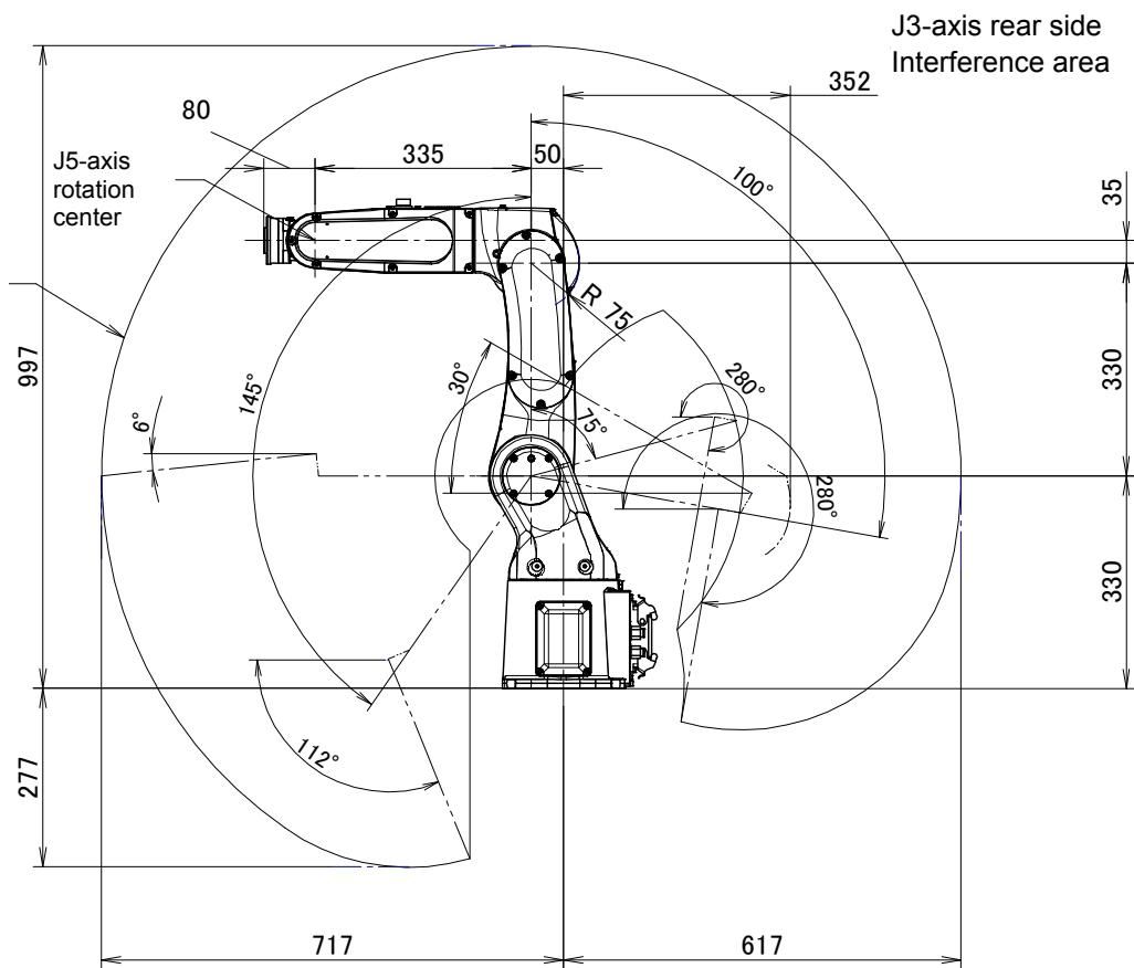
» If applied load on the robot exceeds 5kg when the robot is installed on an angle, the operating area is limited by the mount angle. If payload is less than 5kg, there is no restriction of the operating space.
