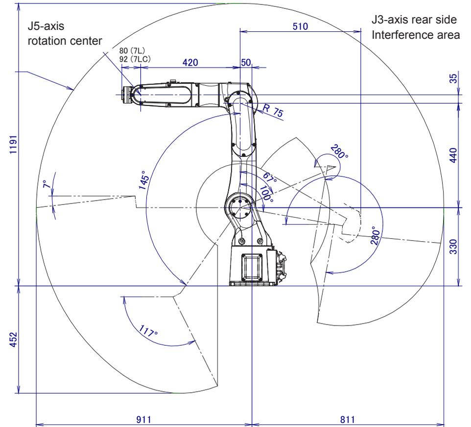
» If applied load on the robot exceeds 5kg when the robot is installed on an angle, the operating area is limited by the mount angle. If payload is less than 5kg, there is no restriction of the operating space.
